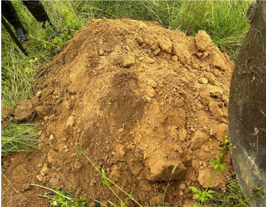
Photo 11 - Typical TOPSOIL unit - brown Silty SAND (TP I)
