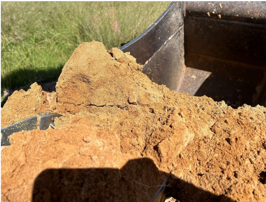
Photo 14 - Clayey SAND observed 2.2m below ground surface (TP E)
