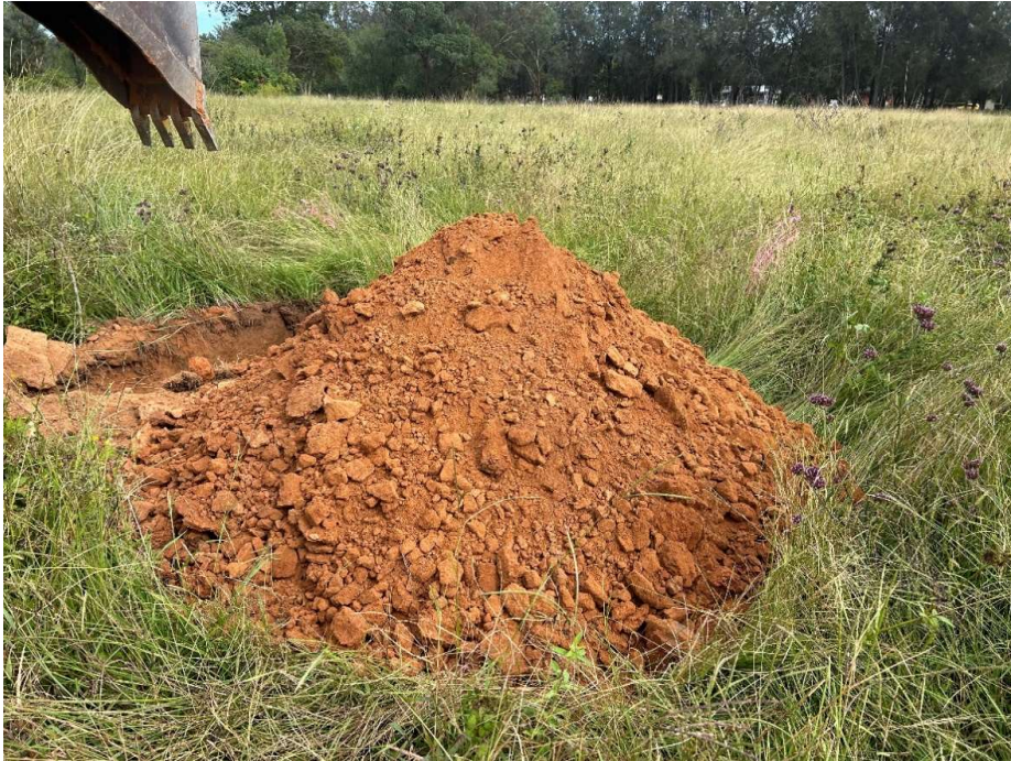
Photo 13 - Typical UPPER INTERBEDDED CLAY unit - Red Brown mottled Grey CLAY (TP H)
