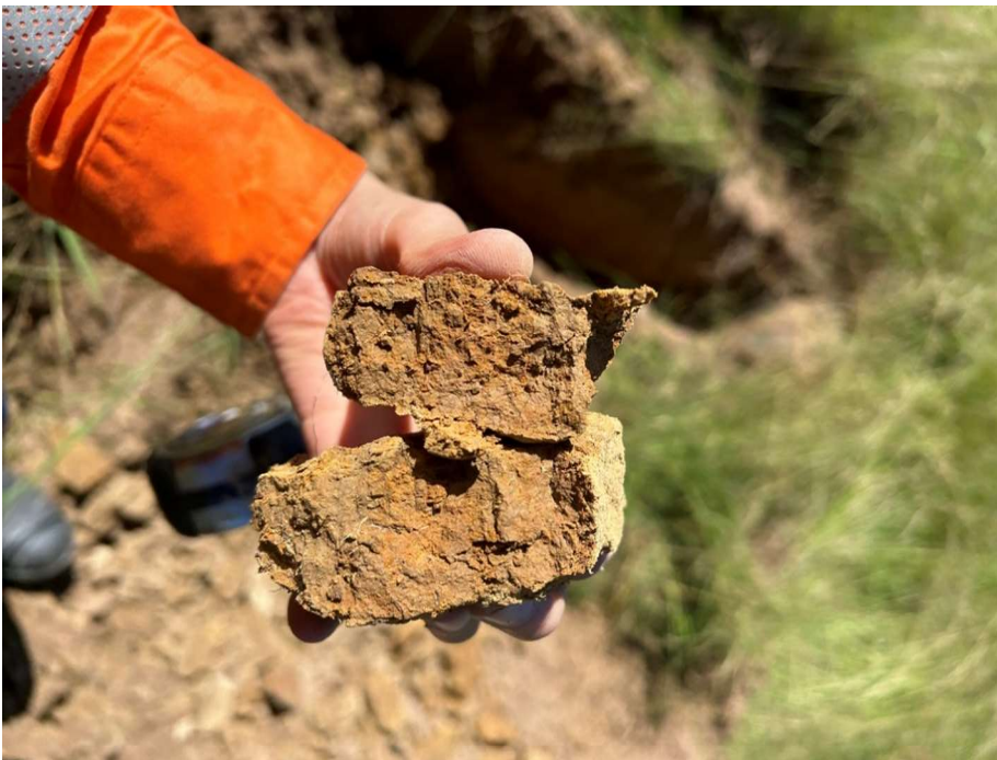
Photo 12 - Typical SURFICAL MATERIAL unit - Yellow Brown CLAY (TP E)
